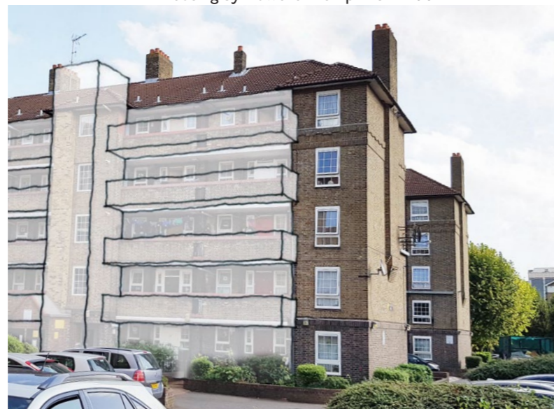
Example sketch view of Montrose access deck infilled to create larger kitchens and bathrooms and new access decks added.
